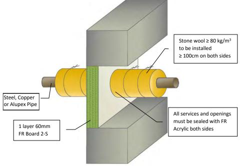
Smoke-safe (<0.1m<sup>3</sup>/h smoke leakage at 200Pa)
